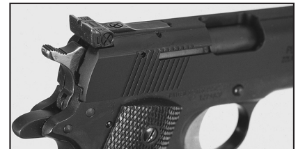
A Millett Gold Cup target rear sight is fitted to the raised, serrated flat-top rail and has adjustments for windage and elevation.
