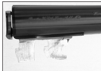
Lock-up is in the Purdy double under-lug fashion. Beretta refers to this system as "progressive," which reflects the slight angle machined into the engagement surfaces. This arrangement keeps the side-by-side's lock-up tight, even as parts wear.
